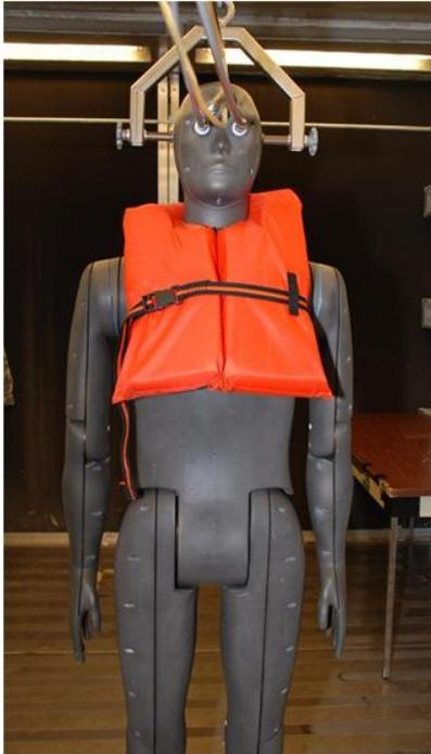
**Figure A6** Kent Sporting, Near Shore Buoyant Vest, Type II PFD
